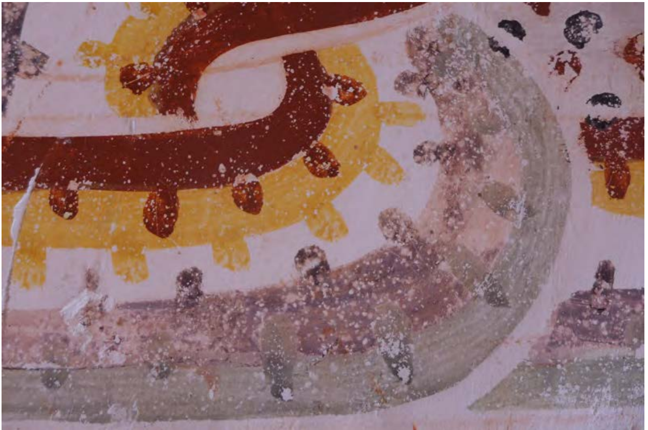
Figure 29. The pink paint layer appears to have altered to a purply black
